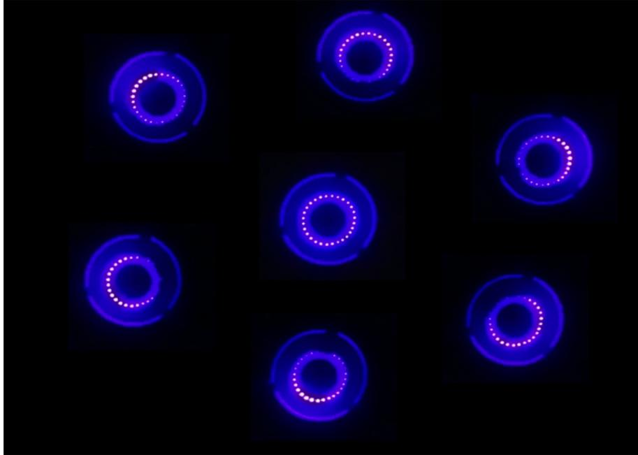
**Figure 5: Superposition of optical images of the ion emitter at different thrust vector angles, and with zero offset in the center**
