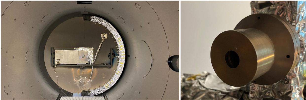
**Figure 4: FOTEC's LIFET-4 with moveable plasma diagnostic arm (left) and a digital Faraday cup (right)**
