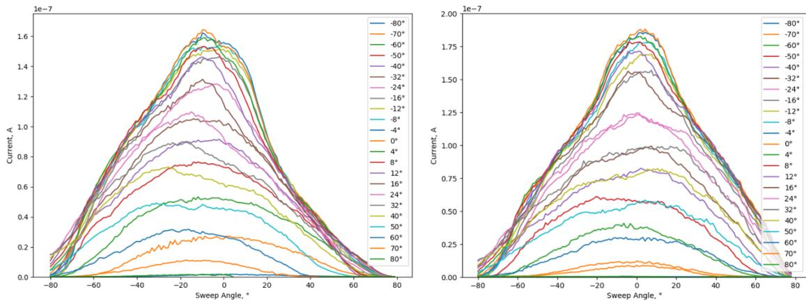
**Figure 6: FC measurement raw data at an operational point of 300  $\mu\text{N}$  with an inclination of 10° and an azimuthal angle of 210° (left) and with an inclination and azimuthal angle of 0° at 350  $\mu\text{N}$  (right)**
