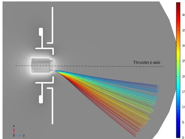
**Figure 2: Simulation of the ion emission of a single needle**
