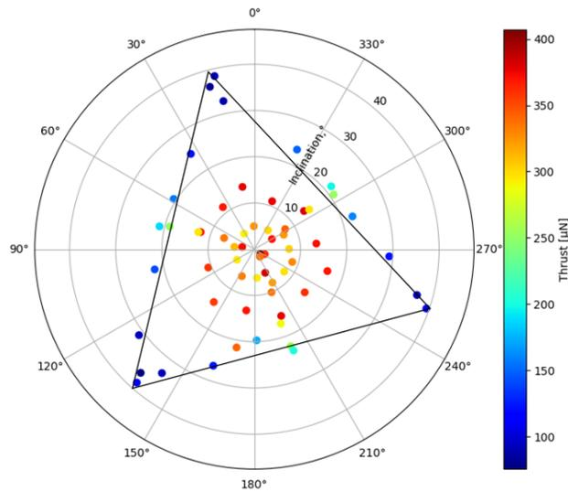
**Figure 9: Measured thrust vectors and thrust levels at various operational points**
