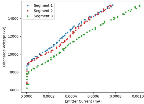
Figure 7: I-V curve for each single extractor segment
