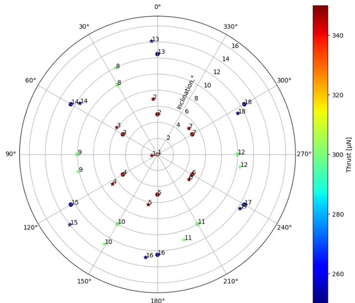
**Figure 10: Measured (stars) and commanded (circles) thrust vectors as well as thrust levels at different operational points, data labels indicate the test number**
