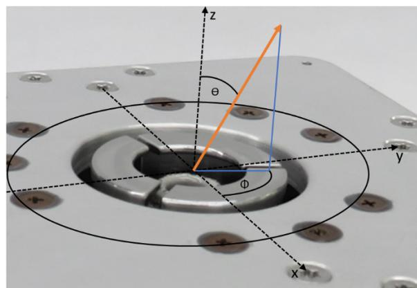
**Figure 3: Spherical coordinate system aligned with the Cartesian system of the thruster**
