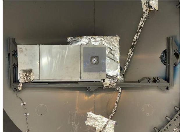
Figure 5: NANO R<sup>3</sup> QM on thrust stand at FOTEC
