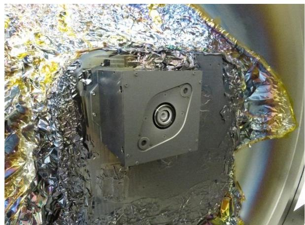
Figure 11: QM installed in TVAC chamber at ENPULSION
