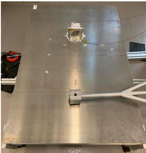
Figure 9: Shock table with installed NANO R<sup>3</sup> QM
