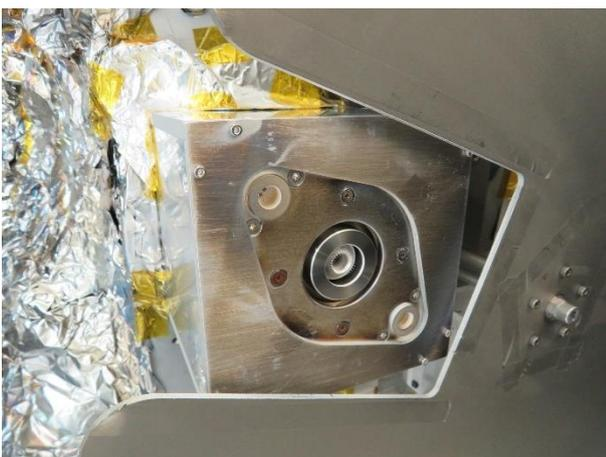
Figure 4: NANO R<sup>3</sup> QM installed in performance test chamber at ENPULSION
