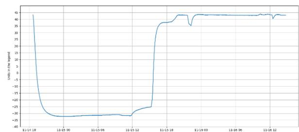
Figure 12: TRP temperature profile for one cycle; jumps in temperature related to change in operational status of thruster
