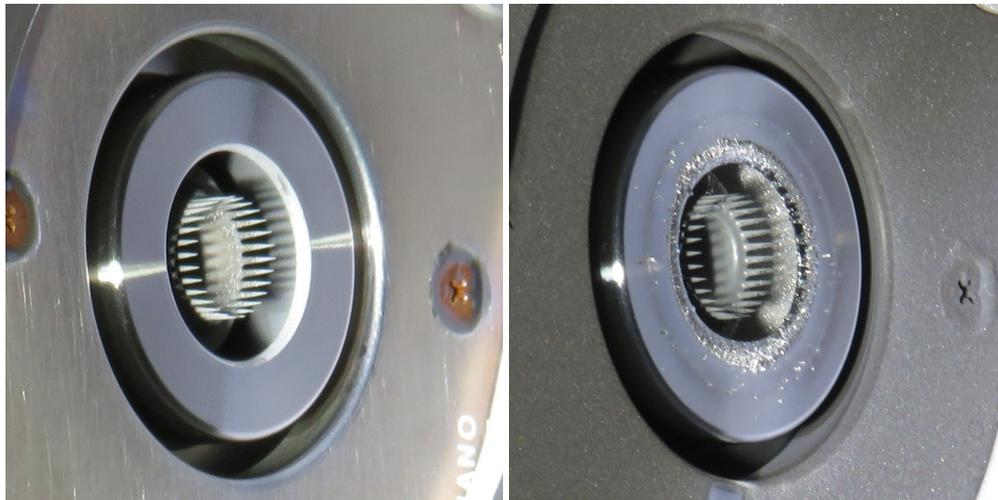
**Fig. 9 Thruster after 0h (left) and 500h (right) of operation at high emitter current for a low mass efficiency emitter. Note the closing of the gap between extractor and emitter**
