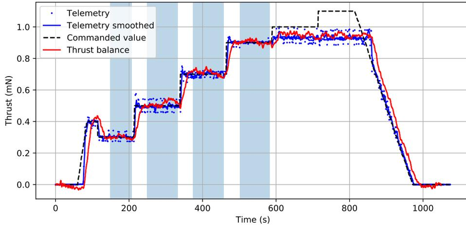
**Fig. 16** Typical thrust response for thrust controlled firing at constant extractor voltage. This corresponds to -7 kV extractor voltage (approximately 3700s specific impulse). Highlighted areas show when the thrust balance is stable.
