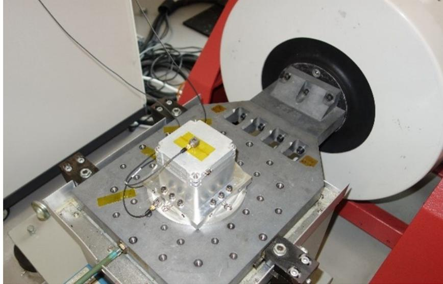
**Fig. 5 NANO R<sup>3</sup> QM mounted on FOTEC shaker**
