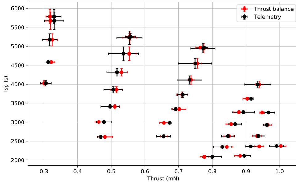
**Fig. 18 Operational map showing difference between calculated and measured thrust for various calculated specific impulses. Specific impulse will depend on exact emitter selection.**
