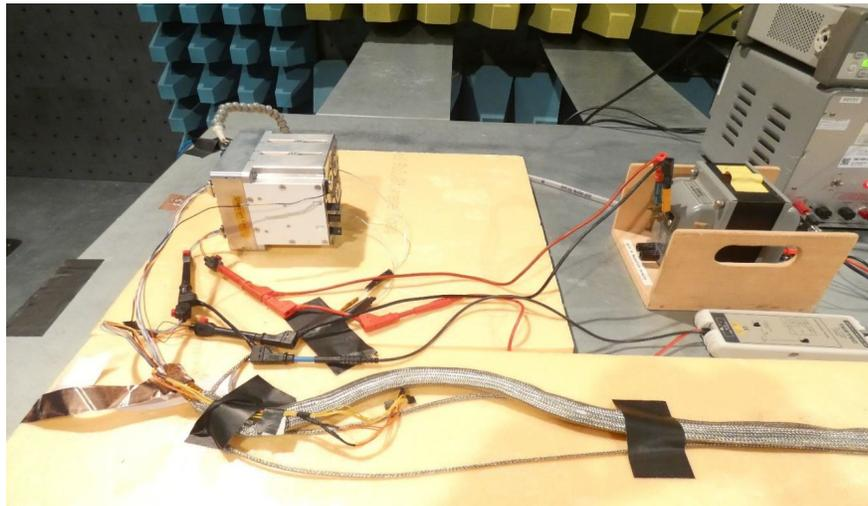
**Fig. 15 MICRO R<sup>3</sup> test setup for conducted susceptibility EMC test**
