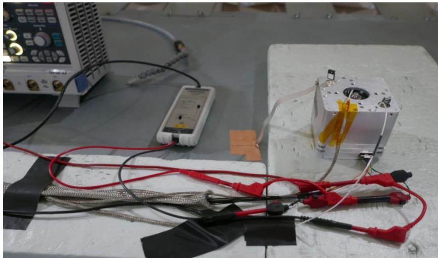
**Fig. 11** Test setup for EMC for the NANO R<sup>3</sup> thruster. The PPU is mated to a dummy thruster model.
