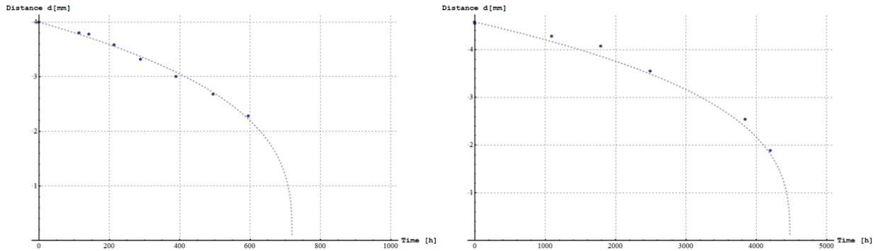
**Fig. 10** Distance between emitter and extractor over time. These plots show the match between experiments (dots) and model (dashed line) for a low mass efficiency emitter operated at higher high current (left) and a high mass efficiency emitter operated at low current (right)
