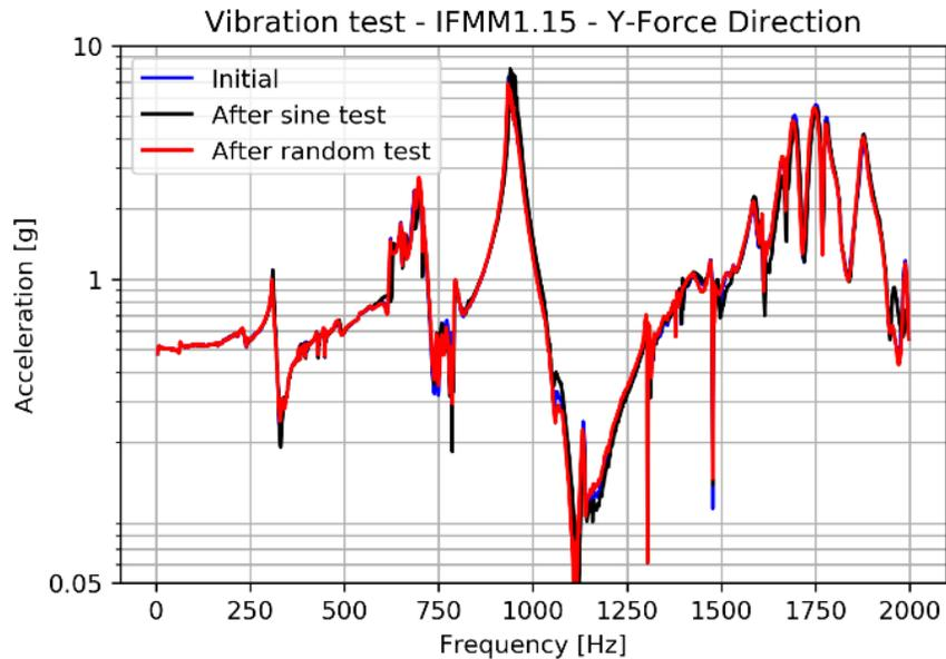
**Fig. 13 Result of resonance sweeps for the MICRO R<sup>3</sup> QM vibration testing**
