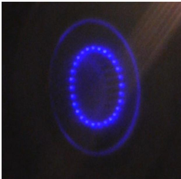
**Fig. 3 NANO R<sup>3</sup> QM firing with full neutralization**
