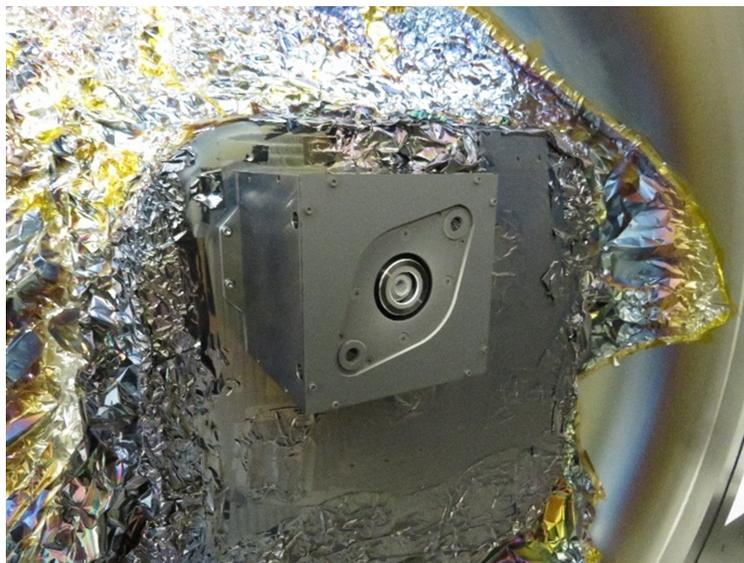
**Fig. 8 NANO R<sup>3</sup> thruster mounted in its TVAC test setup**
