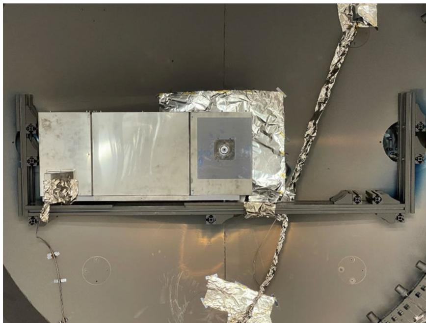
**Fig. 4 NANO R<sup>3</sup> QM mounted on FOTEC's thrust stand**
