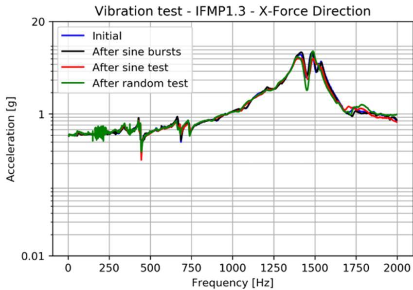
**Fig. 6 Resonance sweep results for vibration qualification of the NANO R<sup>3</sup> QM**
