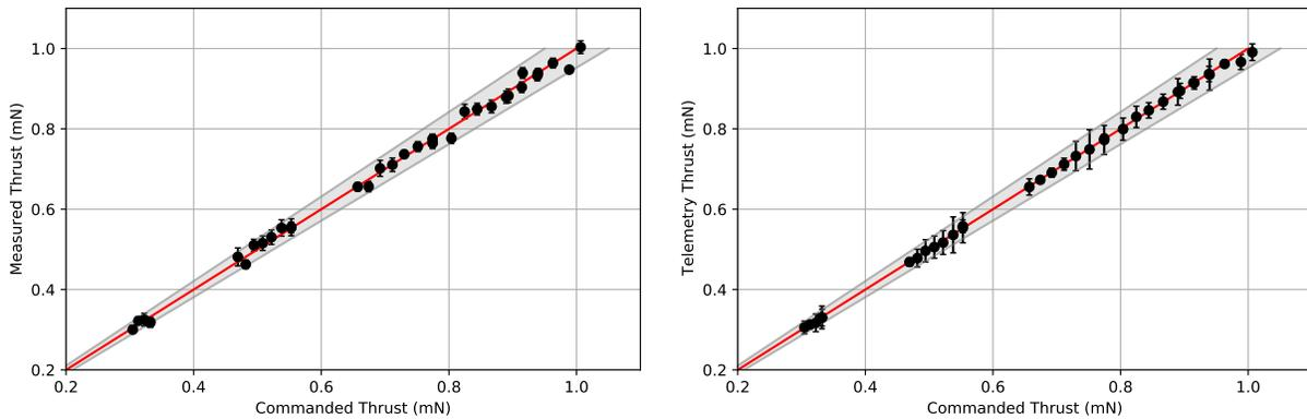
**Fig. 17** Comparison of measured thrust (left) and calculated thrust (right) with commanded thrust, red line represents a 1 to 1 ratio, the grey area represents a 5% error envelope.
