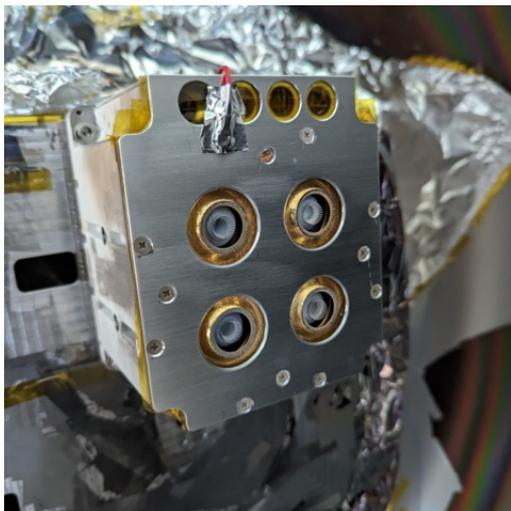
Figure 7. Micro R<sup>3</sup> engineering model equipped with novel extractor design to enhance cleaning capability during subcomponent validation testing
