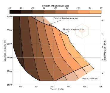
Depending on available power, the user can choose from any operational point. Performance model is shown for 12 V configuration.
