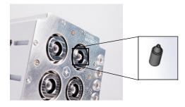
4 Emitters, reservoir for 1.3 kg of indium in a 14x12x10 cm envelope Each emitter is identical to used in the ongoing lifetime test (>30,000 h)
