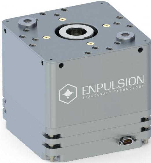
While the required power to operate the *IFM NANO Thruster COTS+* starts at around 8 W, at higher power levels one can choose between high thrust and high specific impulse operation. The *IFM NANO Thruster COTS+* can operate at an  $I_{sp}$  range of 2,000 to 6,000 s.
