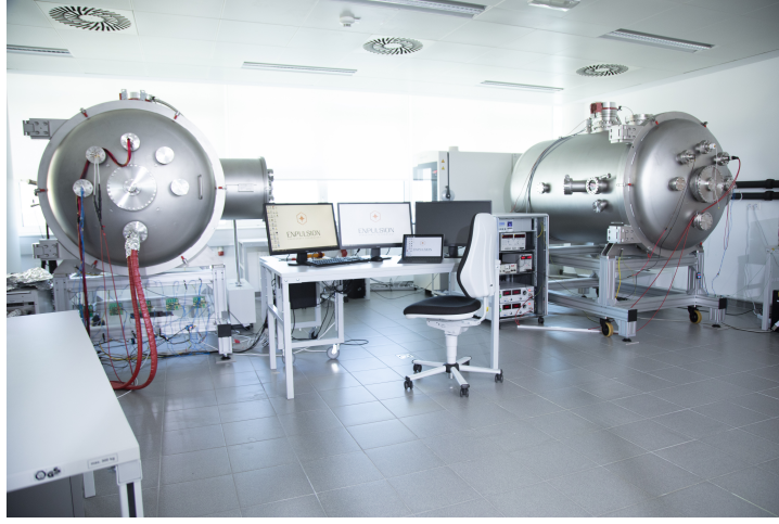
Figure 6: Vacuum chambers for acceptance testing
